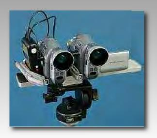
Align two cameras with a specially made rig and record the scene
