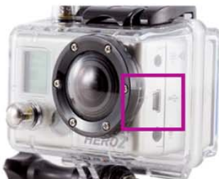
Casing prevent use of USB socket when inside it!
